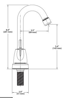
The use of aerator part 116711 reduces flow to a maximum of 1.5 gpm (5.7L/min.)
