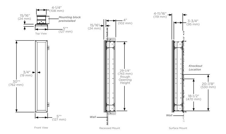
\*Lens dimensions are 1/8" (3 mm) smaller than light body
