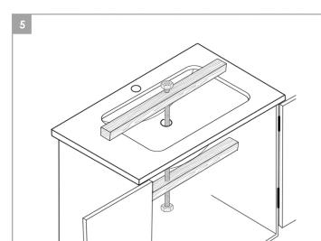
Clamp the sink and hold in place while adhesive cures. There are different methods, we suggest using a couple of pieces of wood with a threaded rod. Set one piece of wood under the sink and another over the countertop.
