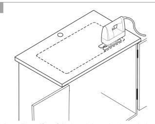
Trace the outline of the template and cut countertop according to templated outline using appropriate cutting tools. Template is for guide only. Use physical sink to ensure accurate cut-out opening. It is recommended to use the actual sink dimensions to ensure the most accurate cut out. Drawing or template are for reference.
