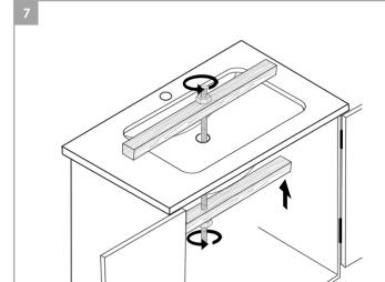
Tighten the clamps to bring the sink up to the countertop. Check the sink's positioning again. Adjust it before the caulk solidifies. When you're satisfied with the sink's placement, leave it clamped in place so the caulk has a chance to cure.
