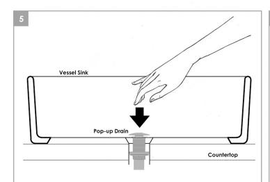
Position sink on countertop and align vessel drain hole with countertop hole and install pop-up drain which also works as an anchor to hold vessel in place.
