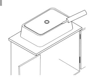
When sink is ready to be installed, put sink up side down and apply a bead of silicone on the outer channel of the sink vessel, alternative use plumber's putty cord.
