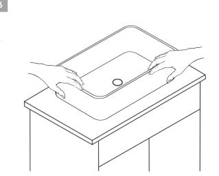
Push down on vessel and ensure is stable and not rocking on countertop. Wipe and clean any silicone excess around the sink bottom.
