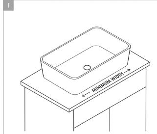
Position sink vessel on the installation surface and confirm vessel size is correct and don't interfere with faucet Note: See minimum countertop space required depending of the model.
