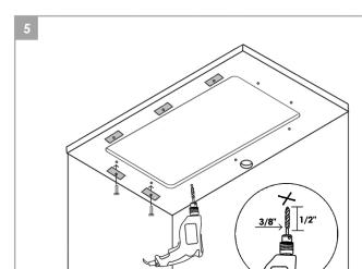
Drill holes on the underside of the countertop, approximately 1/2" from edge of the sink to be installed. Holes should be evenly spaced approximately 6" to 8" apart starting from every corner as shown below.
