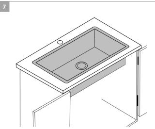
Check alignment of sink again and tighten fasteners to secure sink. Wipe away excess silicone caulk with damp cloth. Connect drain and water supply according to manufacturer's instruction.
