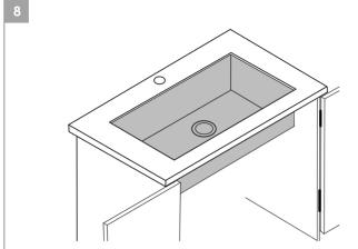
Check alignment of sink again and tighten fasteners to secure sink. Wipe away excess silicone caulk with damp cloth. Connect drain and water supply according to manufacturer's instruction.
