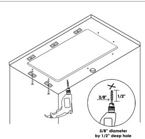
Drill holes on the underside of the countertop, approximately 1/2" from edge of the sink to be installed. Holes should be evenly spaced approximately 6" to 8" apart starting from every corner as shown below.
