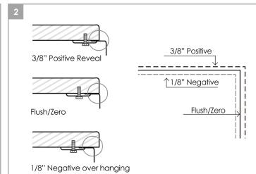
Use scissors to cut along the line of the paper template for you desired reveal type (Negative, Positive or Flush Reveal)
