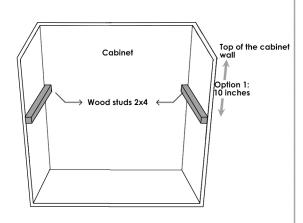
Cut your 2x4 to size and install on the left, right wall of the cabinets, ensure they are leveled and allow space for doors.
