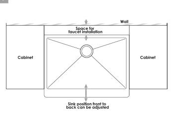
Rest your sink on the supports and check if it is level and flush. For the position front to back, Stylish sinks have a side faces that are full cover, so sink position can be adjusted to leave good space for faucet installation.
