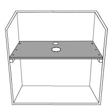
If the width of the cabinet is too large you need to add plywood shelf on top of the 2x4, so the position of the 2x4 should be lower and offset by the thickness of the shelf, in this case is recommended to add a 2x4 at the rear of the cabinet, also shelf will need to have cut-outs to clear the plumbing hoses and drain connections.
