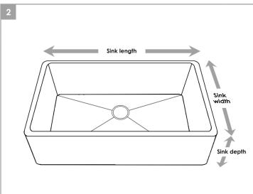
With physical sink present, take dimensions as shown below, you will measure the length, depth, and width and make sure is compatible with your cabinet size.
