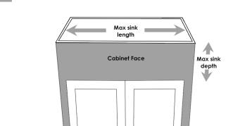
Cabinet size: Minimum cabinet internal opening (left to right) should be 1/4 inch larger than sink length
