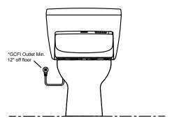
\*The 3-prong cord on the Washlet is on the right side and is 4' long. The GFCI outlet needs to have120V, 10amps.
