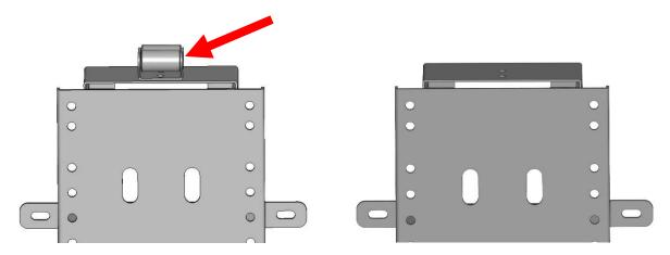
2. Once the roller is removed, install the flat top lid mount to the adjustable top bracket with the screws provided with the lid mount.
