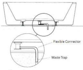
Figure 2 Flexiable connector installation \*\*\* Flexiable connector and waste trap are not supplied
