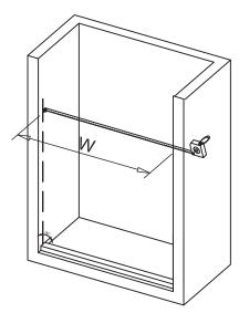
2. Your Upper Guide Rail [5] and Bottom Guide Rail [9] have been precut for your Shower model opening width, eg.60" for shower width. If W-width of your wall-to-wall opening is equal to the size of your Shower model, it is unnecessary to cut the Upper Guide Rail and Bottom Guide Rail and you can continue to Step 3.
