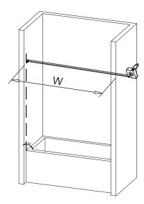
2. Your Upper Guide Rail [5] and Bottom Guide Rail [9] have been precut for your Shower model opening width, eg.60" for shower width. If W-width of your wall-to-wall opening is equal to the size of your Shower model, it is unnecessary to cut the Upper Guide Rail and Bottom Guide Rail and you can continue to Step
