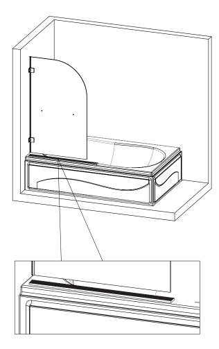
Pleae prepare a long slat 1000x30mm @ 10~12mm thickness to hold on the glass panel during the installation.
