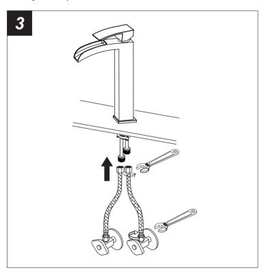
3. Connect the flexible hoses to water supply valve (not included) and copper tubes, and tighten it with adjustable wrench. **DON'T OVER TIGHTEN!**
