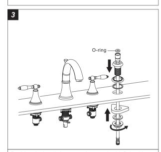
Position the hand shower and secure it with fixing kit.
