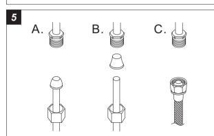
Connect to water supply lines with either:
