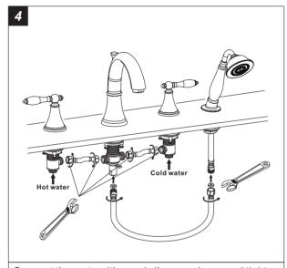
Connect the parts with supply lines as shown and tighten them with wrench.
