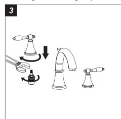
Place a new cartridge in the cartridge seat, tightening the cartridge with a spanner, then screw the handle with hand.
