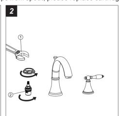
Unscrew the old cartridge② with Adjustable Wrench①, then take it out .
