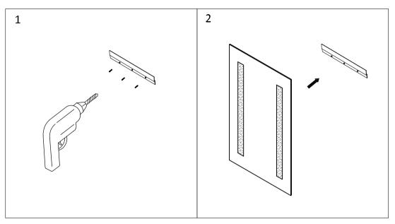
1.Install the hanger by screws on wall, make sure the hanger is stable. 2.Hang the mirror on the hanger.
